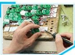
6. Repair welding process
