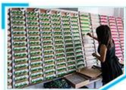
9. Aging test for travel charger
