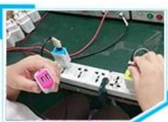
9. Aging test for travel charger
