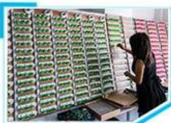
9. Aging test for travel charger
