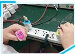
9. Aging test for travel charger
